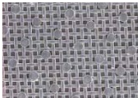
SAATI HiBond Plus halftone area with no stencil loss
