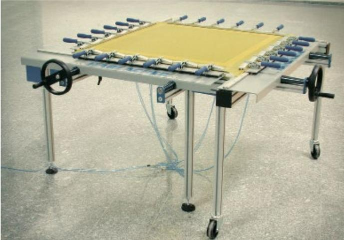
The Harlacher H25-5 is a mechanical stretcher with pneumatic lifting. This sturdy tensioning unit enables you to meet the most demanding tensioning requirements at an excellent price performance ratio.
